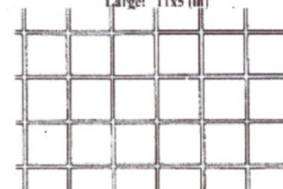
Quarry Tile 2 Sizes 275x275 & 220x220 (mm) or 11x11 & 8.5x8.5 (in)
